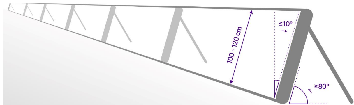
Figure 3. Diagram of the kickboard on the sides of the pitch.
